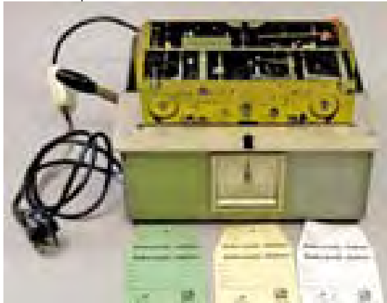
Electromechanical time clock (race timekeeping device) from the company "Württembergische Uhrenfabrik Bürk Söhne, Schwenningen" Type: ZS 67/2s, No. 36673 for 220V AC. This clock was developed for use in public races. The participant's time, measured down to the second, was stamped onto his participant card. Due to unavoidable delays at the start and finish, the stamped time usually exceeded the individual's actual time.
